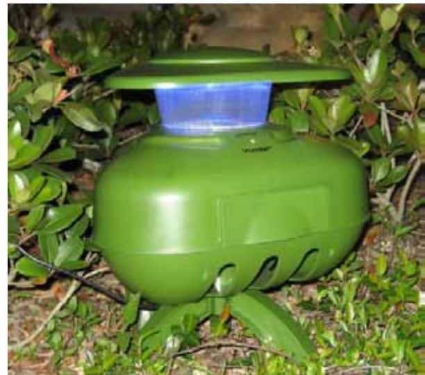
Mosquito Trap with Carbon Dioxide (CO 2 ) attractant
