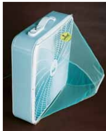
Mosquito Trap, No Carbon Dioxide attractant
